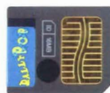
SmartMedia-Card (SMC), a Flash format developed by Olympus and Fuji for mobile equipment. Shown here as game medium for the Korean GP32 handheld (Gamepark, 2001).
