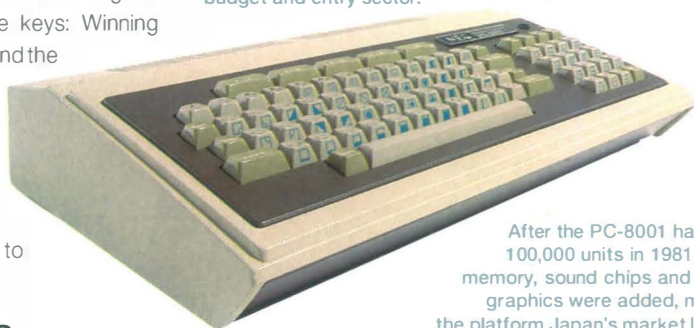
With mini keys, cart slots and joystick ports, the PC-6001 tried the low budget and entry sector.
