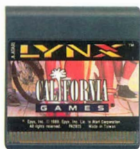
Cards for the Atari Lynx contain 128 to 512 K (Epyx, 1989).
