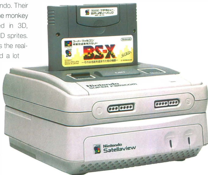
Japanese Nintendo gamers received their programs via satellite. The BS-X adapter contained a small flash cartridge.
