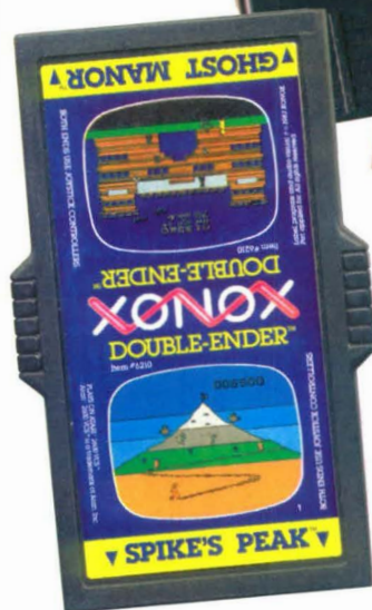
Double Enders' cartridge for the Atari VCS, two times 8 K with connectors on both sides (Xonox, 1983).
