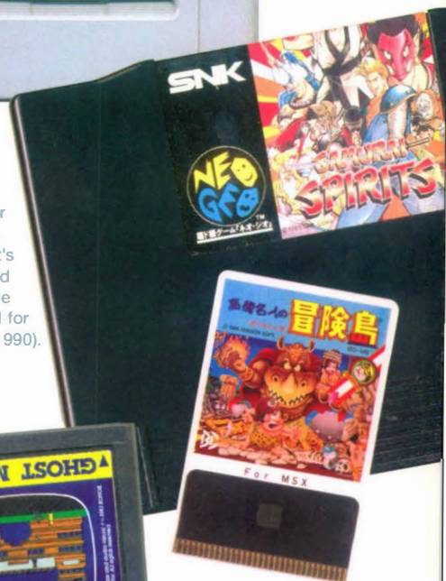
BeeCard is the rare predecessor to the HuCard; MSX computers required a special adapter to read it (Hudson, 1986).
