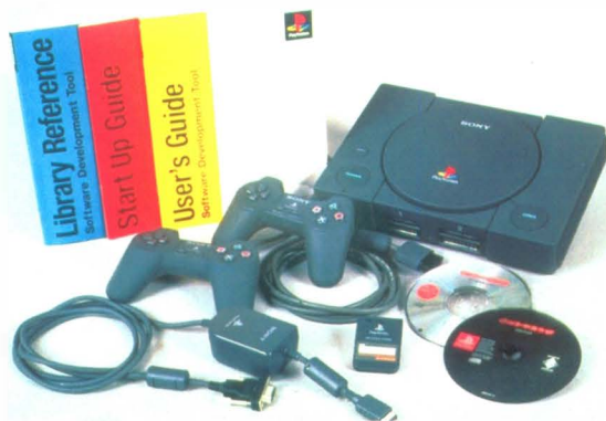
Sony attracted hobby programmers with the dark Net Yaroze console, its PC connectivity and its development tools.
